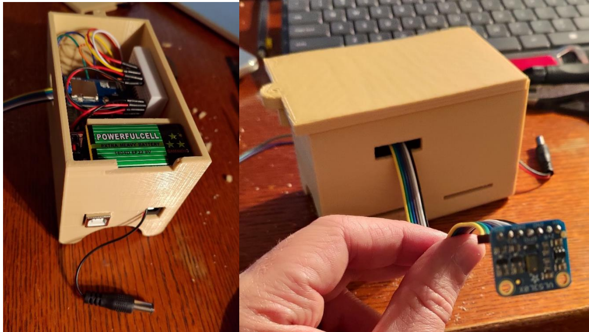
Figure 3: 3D Printed Arduino Suspension Testing Box [2]
